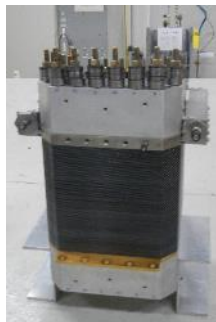
Cell Stack (1,25MW, 250Nm 3 /h)
